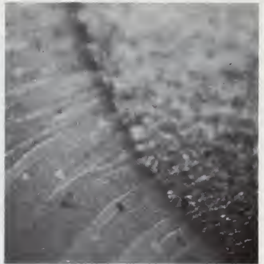
EPON 828 + 2 pph R-151 + 8 pph 20-64 + 5 pph CURING AGENT D (137.5X)
